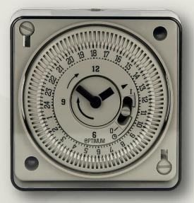
OP-TS111.2 IS A CAPTIVE-TAPPET 24 HOUR TIME SWITCH. EACH TAPPET OPERATES FOR 15 MINUTES. THE TIMER IS SUITABLE FOR PANEL MOUNTING. PANEL CLIPS ARE INTEGRATED INTO THE HOUSING. THE 24 HOUR DIAL CONTROLS A VOLT-FREE CHANGEOVER SWITCH, WITH A RESISTIVE RATING OF 16 AMPERES.
