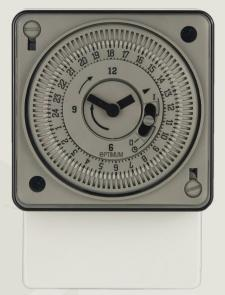
TIME SWITCH. EACH TAPPET OPERATES FOR 15 MINUTES. THE TIMER IS SUITABLE FOR SURFACE, PANEL AND DIN-RAIL MOUNTING. THE 24 HOUR DIAL CONTROLS A VOLT-FREE CHANGEOVER SWITCH, WITH A RESISTIVE RATING OF 16 AMPERES. THERE IS AN INBUILT RE-CHARGEABLE CELL TO KEEP THE TIMER RUNNING IN THE EVENT OF A LOSS OF MAINS POWER.
